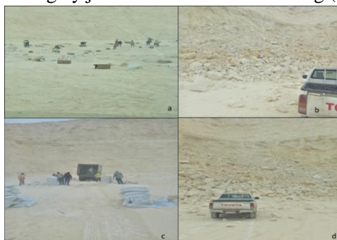
Fig. 4. Blasting trial -1 during charging and muck pile fragmentation
