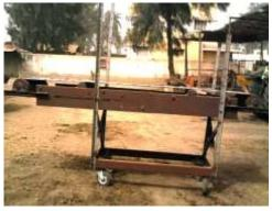
Fig. (3) Photo of the proposed belt conveyor.
