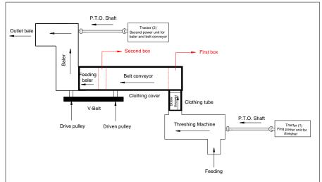
Fig. (1) A schematic diagram of the proposed first-trial baling system
