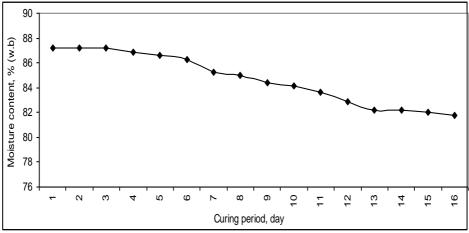
Fig. (2): Change in the average bulbs moisture content as related to curing period in the open field.
