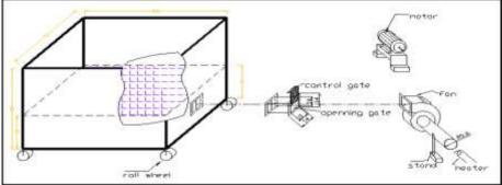
Fig. (1): A schematic diagram of the flatbed batch dryer type.
