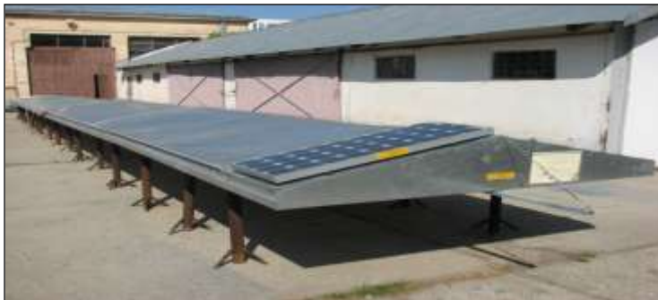
Fig. 3: Solar tunnel dryer in experimental place
