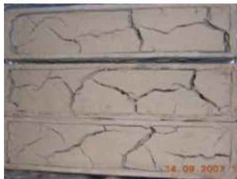
Fig. 8: Shrinkage and cracks for clay samples.
