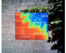
Figure (4) Infrared photography demonstrating temperatures on the building surface.
