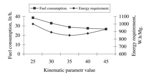
Fig. 5: Effect of kinematic parameter value on fuel and energy requirements at different pile heights
