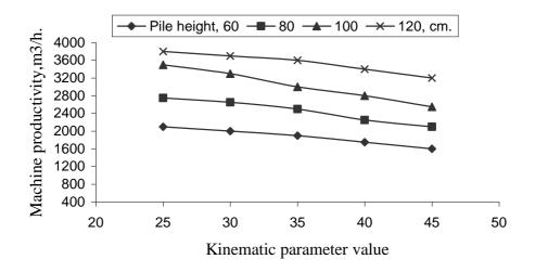
Fig. 3: Effect of kinematic parameter value on machine capacity at different pile heights.
