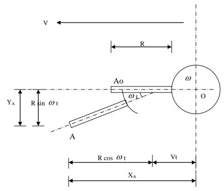
Fig.2 : Kinematics of compost turning machine
