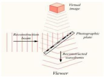
**Fig.4.** Shows the Method of Forming Hologram **Source:** Ramachandiran, C. R., Chong, M. M., & Subramanian, P. (2019)
