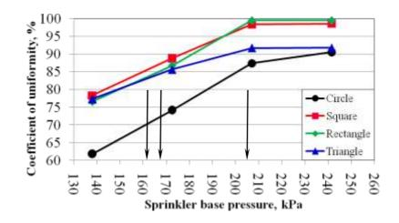
Figure (14): effect of Sprinkler base pressure on coefficient of uniformity for different nozzle shapes.
