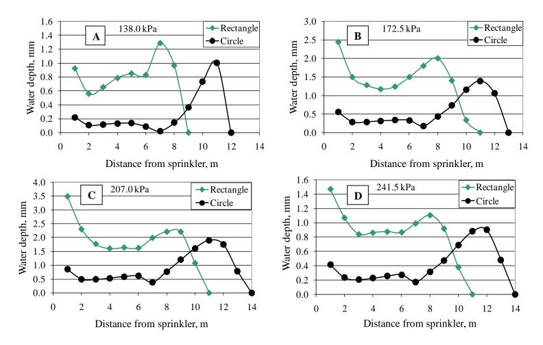
Figure (5): Water application profiles for circle and rectangle orifices at sprinkler base pressure (A) 138.0, (B) 172.5, (C) 207.0 and (D) 241.5 kPa.
