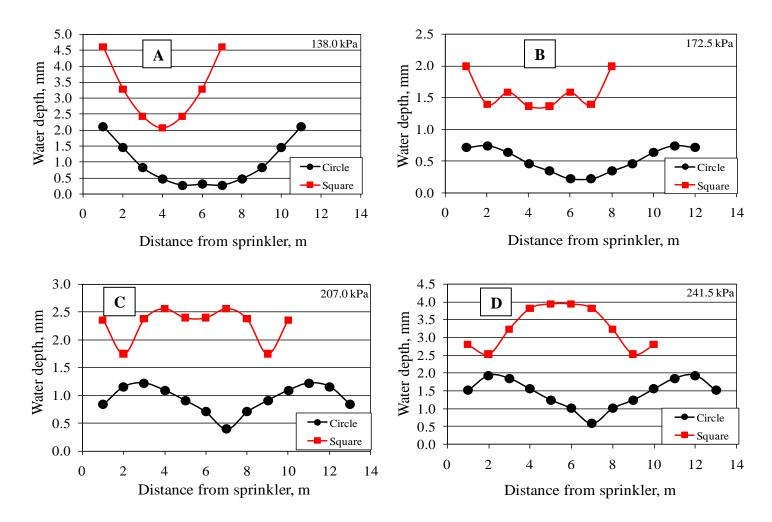
Figure (8): Water application profiles for circular and square orifices with 100% overlapping at sprinkler base pressure (A) 138.0, (B) 172.5, (C) 207.0 and (D) 241.5 kPa.
