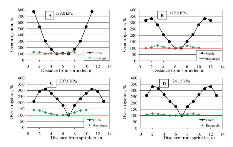
Figure (12): Over irrigation application profiles % for circular and rectangular orifices with 100% overlapping at sprinkler base pressure (A) 138.0, (B) 172.5, (C) 207.0 and (D) 241.5 kPa.
