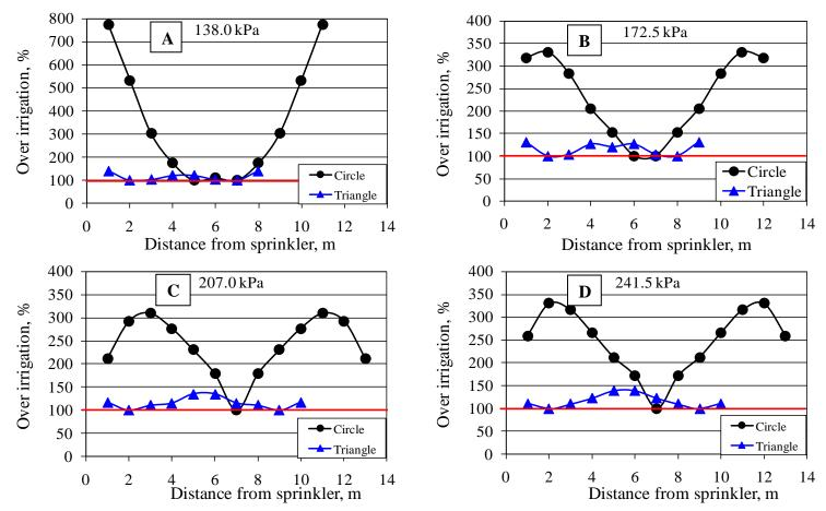
Figure (13): Over irrigation application profiles % for circular and triangular orifices with 100% overlapping at sprinkler base pressure (A) 138.0, (B) 172.5, (C) 207.0 and (D) 241.5 kPa.
