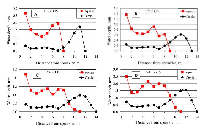
Figure (4): Water application profiles for circle and square orifices at sprinkler base pressure (A) 138.0, (B) 172.5, (C) 207.0 and (D) 241.5 kPa.
