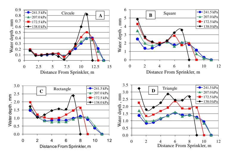
Figure (7): Water application profiles for (A) circle, (B) square, (C) rectangle and (D) triangle orifices at different sprinkler base pressure.
