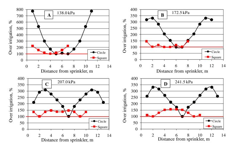
Figure (11): Over irrigation application profiles % for circular and square orifices with 100% overlapping at sprinkler base pressure (A) 138.0, (B) 172.5, (C) 207.0 and (D) 241.5 kPa.
