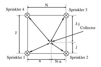
Figure (3): Distance between sprinklers and collectors.
