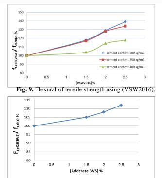
**Fig. 10.** Splitting tensile strength using (addcrete BVS) with (c.c) 350kg/m<sup>3</sup>
