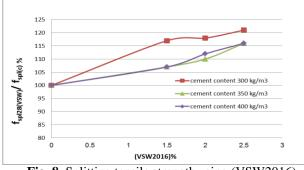
Fig. 8. Splitting tensile strength using (VSW2016).
