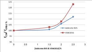
Fig. 7. Drying shrinkage using BVS, (VSW2016) with 350 kg/m<sup>3</sup>.
