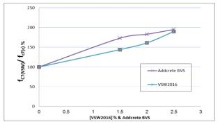
Fig. 5. Compressive strength at 7 days using BVS, (VSW2016) with C.C. 350 kg/m<sup>3</sup>.
