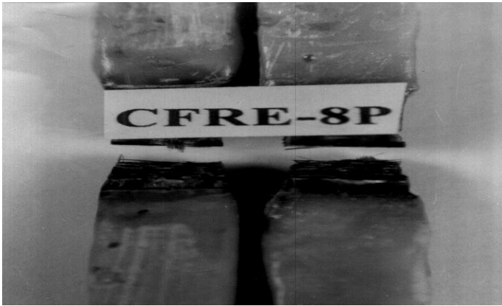
Fig. 5c: Macroscopic Fractograph of Carbon Fiber Composites.
