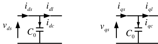
Fig. A1: d-q equivalent circuit of the self excitation capacitor.
