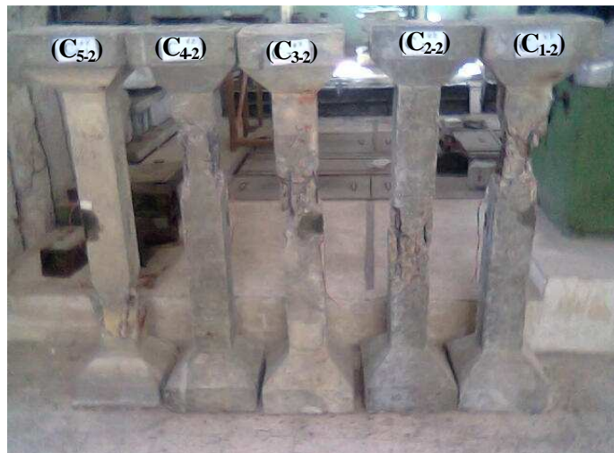
Photo 2: Cracks and mode of failure of R.C. tested columns (Group B)
