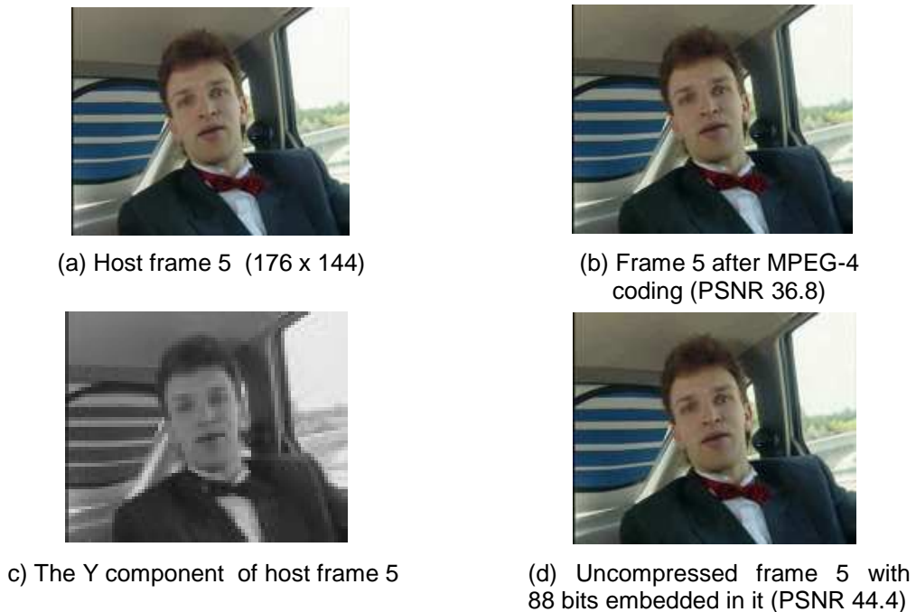
Figure 8: (a) host frame from the car video sequence, uncompressed. (b) Host frame after MPEG-4 encoding (12 frames/second), (PSNR 36.8). (c) The Y component of car video frame 5. (d) Frame 5 without MPEG encoding with 88 bits embedded in it (PSNR 44.4).
