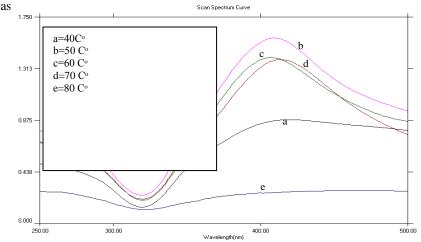
Reaction conditions: Honey, 1ml and AgNO<sub>3</sub>, • 0.1 m mole/100 ml water; pH11.; time 60 min. Fig. 3. Effect of temperature on the formation of silvr nano particales.
