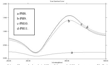
Reaction conditions: Honey, 1ml and AgNO3,  $\star$  0.1 m mole/100 ml water , temp 50 °C; time 60 min.
