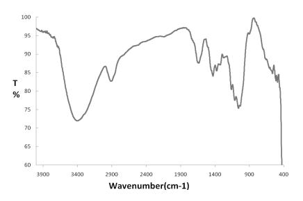
Fig. 3c. FTIR spectrum of paperboard coated by WP/PVA/glycerol blend .
