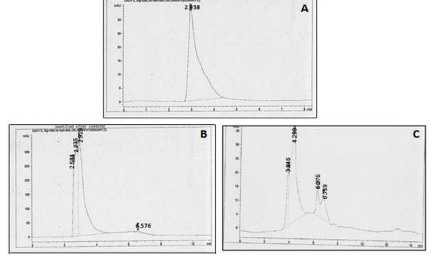
**Fig. 1:** HPLC Chromatogram of (A) Standard Warfarin, (B) Warfarin-intoxicated postmortem blood sample, and (C) Control postmortem blood sample.
