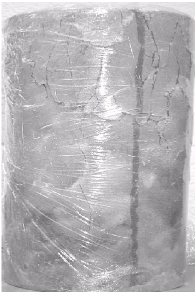
Cone and split failure
