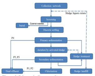
Figure 2. Schematic diagram of wastewater treatment processes used in studied units.
