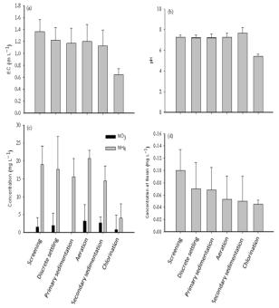
Fig. 4. Efficacy of different processes used at wastewater treatment plants for the removal of salinity (a), acidity (b), NO<sub>3</sub> & NH<sub>4</sub> (c) and B (d).
