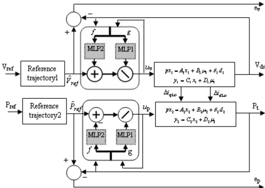
Fig. (4) : Block diagram of the wind energy conversion system with the proposed NARMA-L2 controller.
