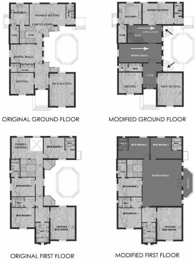
FIGURE - (5) STRUCTURAL FLEXIBILITY (EXTENDABILITY)
