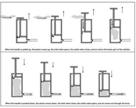
Figure 3. An illustration of How a Tire Pump Works (Mayer, 2014)
