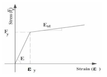
Fig. 1 Idealized Stress-strain curve for steel
