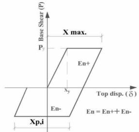
Fig. 6 Lateral drift- Base shear relationship (Max. excursion)
