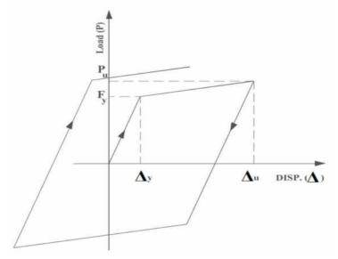
Fig. 4 Load-Displacement relationship for cyclic loading
