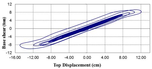
Fig. 8 Lateral drift-base shear relationship for the frame 1, Considering SUMATRA EQ. at P.G.A, 0.35G
