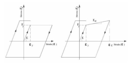
(a) Perfectly Plastic Cyclic Model (b) Strain Hardening Cyclic Model Fig. 2 Perfectly Plastic and Strain Hardening Cyclic Model Where,  $f_s$  is the steel stress;  $f_y$  is the specified yield strength of steel;  $\varepsilon_s$  is the steel strain and  $\varepsilon_y$  is the steel yield strain.
