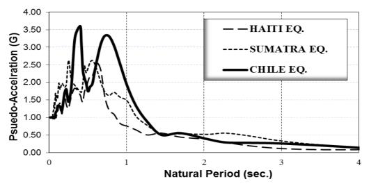
Fig. 5 Response spectra for earthquake records
