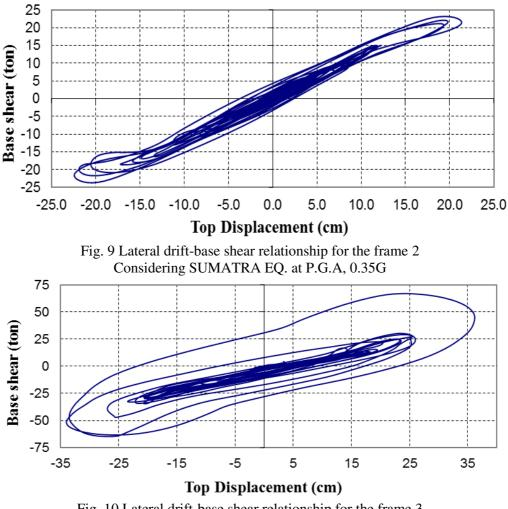
Fig. 10 Lateral drift-base shear relationship for the frame 3 Considering SUMATRA EQ. at P.G.A, 0.35G
