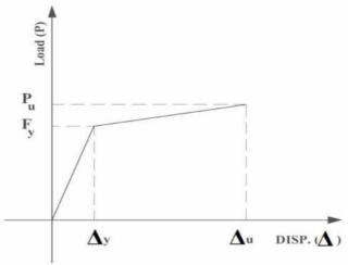
Fig. 3 Load-Displacement relationship for monotonic loading
