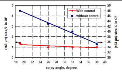
Fig. 5: Effect of spray angle value on the percentage of +63 µm separated in the overflow
