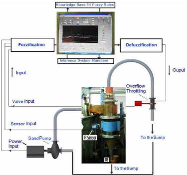
Fig. 3: The generic structure of the fuzzy hydrocyclone control
