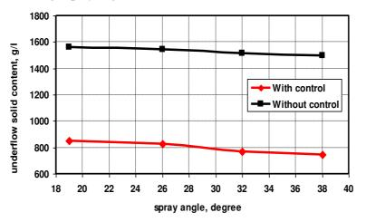
Fig. 7: Effect of spray angle on the underflow solid content
