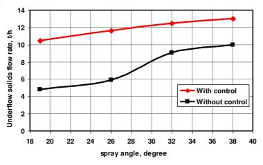
Fig. 8: Effect of spray angle on the underflow solids flow rate
