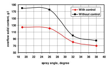
Fig. 6: Effect of spray angle on the overflow solid content
