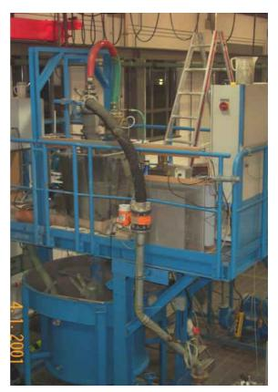
Fig. 1b: Photo of semi-technical controlled hydrocyclone plant
