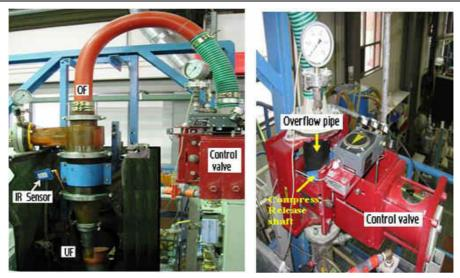
Fig. 2: A 150 mm Hydrocyclone with IR sensor and a control valve around the overflow pipe
