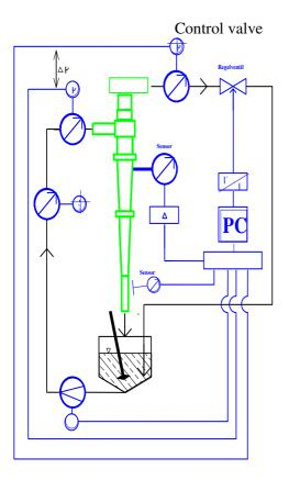
Fig. 1a: Flow chart of semi-technical single controlled hydrocyclone plant
