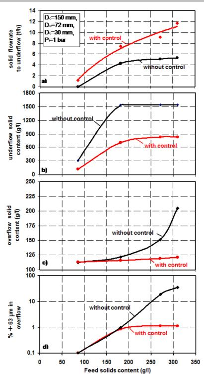
Fig. 9: Classification of sand/kaolin mixture with and without control at spray angle of  $26^{\circ}$
