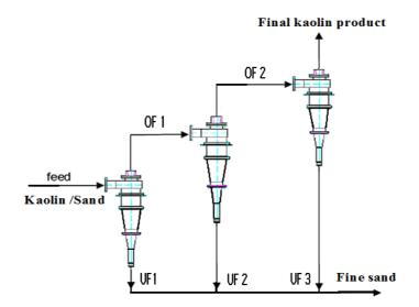
Fig. 4: Kaolin processing using multistage hydrocyclone separation
