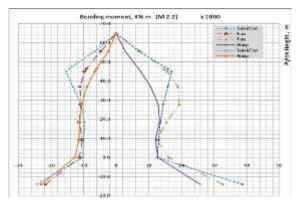
Fig.10. Tower lateral bending moment extreme values (beside hinged support)
