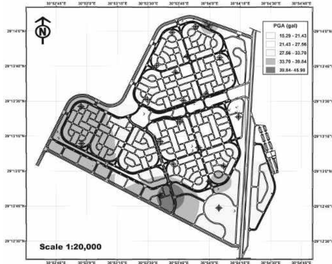
Fig. 12. Distribution of peak ground acceleration (PGA) at ground surface
