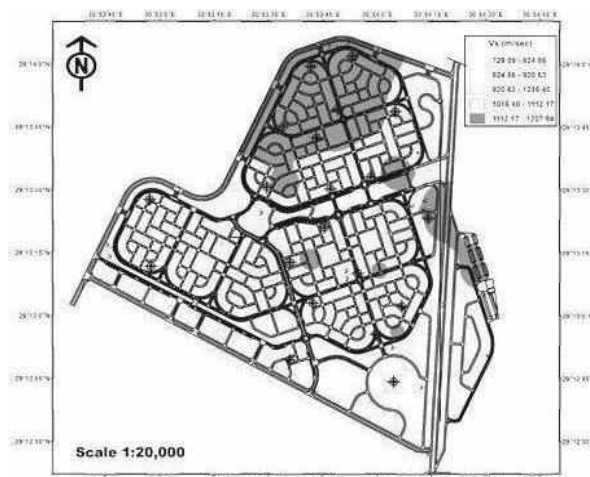
Fig. 11. The average shear wave velocity distribution in El-Fayoum New City
