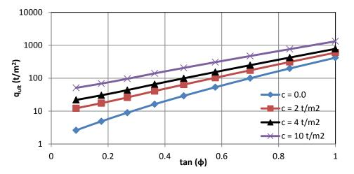
Fig. 6 .Ultimate bearing capacity versustan  $\emptyset$  at  $R_f = 1$  for different values of c
