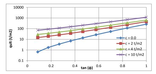
Fig. 5. Ultimate bearing pressure versustan  $\emptyset$  at  $R_f = 0.0$  for different values of c
