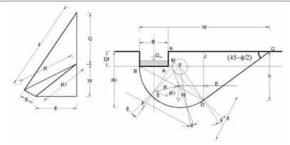
Fig. 1. Failure mechanism, according to Krey's method (after [5])
