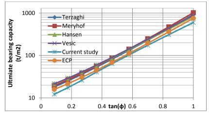
**Fig. 12.** Ultimate bearing capacity versus  $\tan \emptyset$  at B = 1.0 m, Rf = 1, c = 2 t/m<sup>2</sup> using different methods
