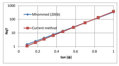
Fig. 13. Bearing capacity factor  $(N_{q\gamma})$  versus tan  $\varphi$  at  $R_f = 0.0$  for Mohammed [15] and current method s
