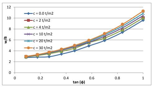
Fig. 10. Maximum extent of failure surface (w/B) versus  $tan(\phi)$  at  $R_f = 0.0$  and B = 2 m for different values of c
