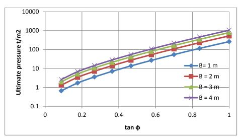
Fig. 3. Ultimate bearing capacity versustan  $\emptyset$  at  $R_f = 0.0$  for different values of B
