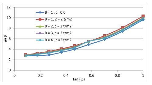
Fig. 9. Maximum extent of failure surface (w/B) versus tan ( $\phi$ ) at  $R_f = 0.0$  for different values of c and B
