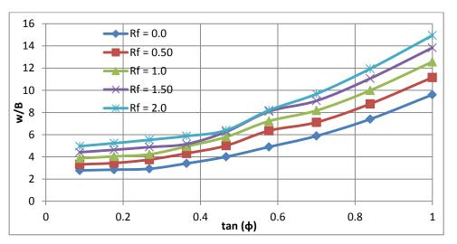
Fig. 7. Maximum extent of failure surface (w/B) versus  $tan(\phi)$  at c = 0.0 for different values of  $R_f$
