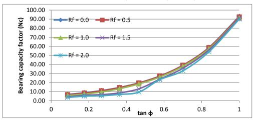
Fig. 11. Bearing capacity factor ( $N_c$ ) versus tan  $\varphi$  for different Rf
