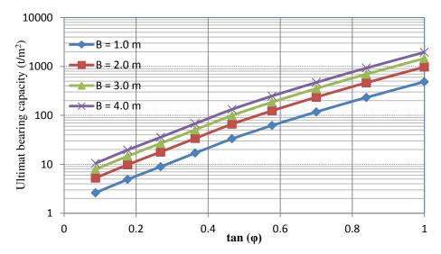
Fig. 4. Ultimate bearing capacity versustan  $\emptyset$  at  $R_f = 1.5$  for different values of B
