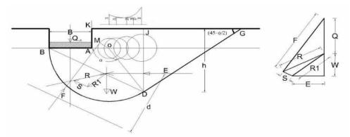
**Fig. 2.** Determination of ultimate bearing capacity force Q<sub>ult</sub> using Krey's method (friction circle method)
