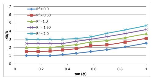
Fig. 8. Maximum depth of failure surface (d<sub>o</sub>/B) versus tan ( $\phi$ ) at c = 0.0 for different values of R<sub>f</sub>
