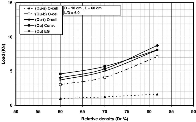
Figure 10. Ultimate load-relative density relationship (D=10cm, L/D = 6 )
