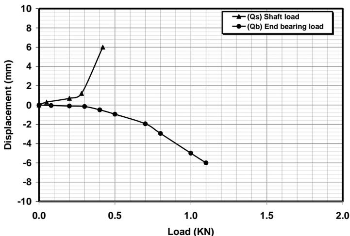
Figure 4. Load-displacement relationship (O-cell tests,  $D_r = 70\%$ ,  $D=6\text{cm}$ ,  $L/D = 10$ )
