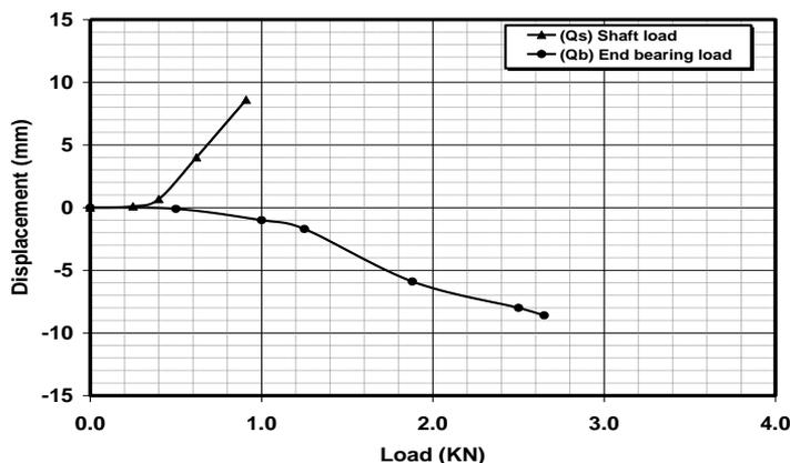
Figure 5. Load-displacement relationship (O-cell tests,  $D_r = 70\%$ ,  $D=8.6\text{cm}$ ,  $L/D = 7$ )
