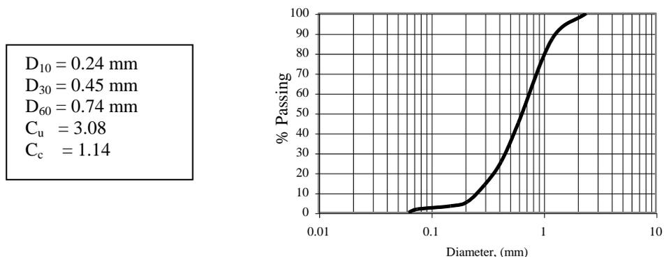
Figure 3. Grain size distribution curve for the tested sand soil
