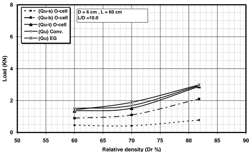
Figure 8. Ultimate load-relative density relationship (D=6cm, L/D = 10 )
