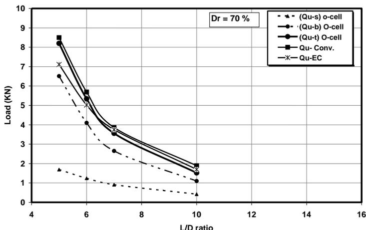
Figure 12. Ultimate load -L/D ratio relationship ( $D_r = 70\%$ )
