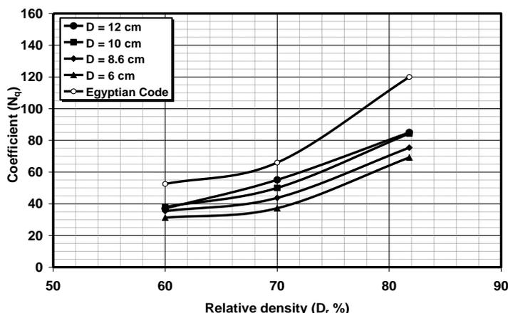
Figure 14. Relationship between coefficient ( $N_q$ ) and relative density (O-cell tests)
