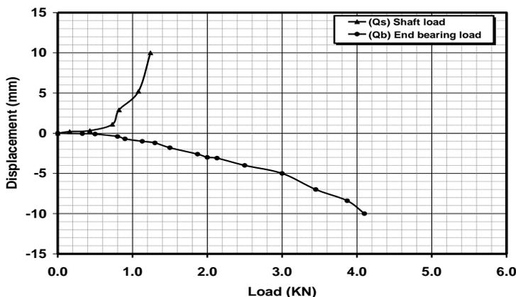
Figure 6. Load-displacement relationship (O-cell tests,  $D_r = 70\%$ ,  $D=10\text{cm}$ ,  $L/D = 6$ )
