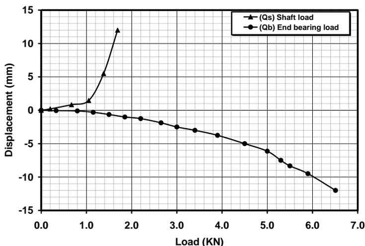
Figure 7. Load-displacement relationship (O-cell tests,  $D_r = 70\%$ ,  $D=12\text{cm}$ ,  $L/D = 5$ )
