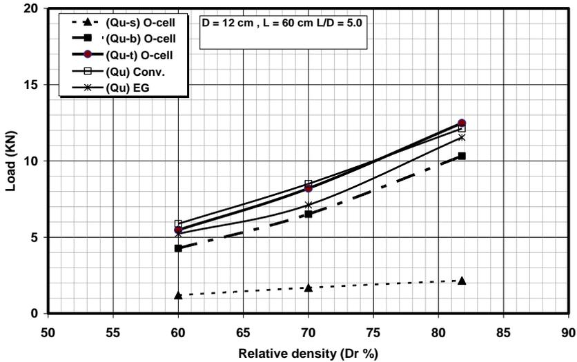
Figure 11. Ultimate load-relative density relationship (D=12cm, L/D = 5 )
