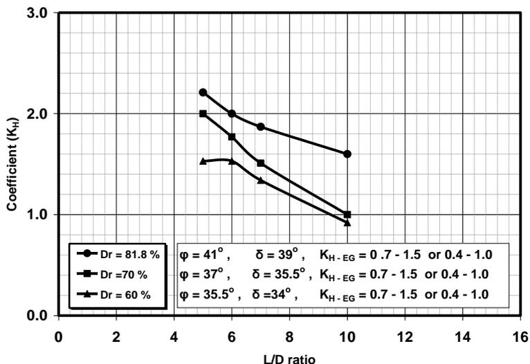
Figure 15. Relationship between coefficient ( $K_H$ ) and L/D ratio (O-cell tests)
