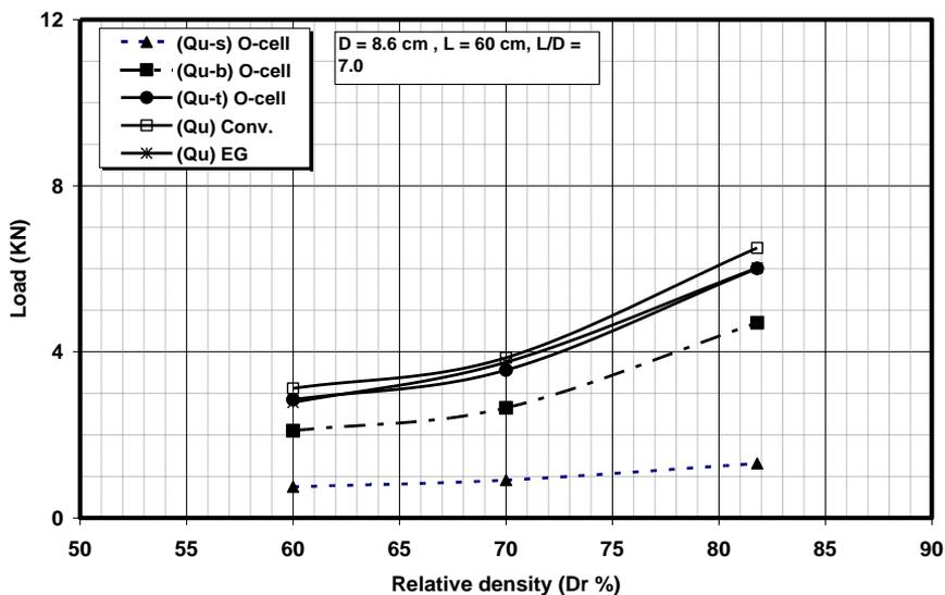
Figure 9. Ultimate load-relative density relationship (D=8.6cm, L/D = 7 )
