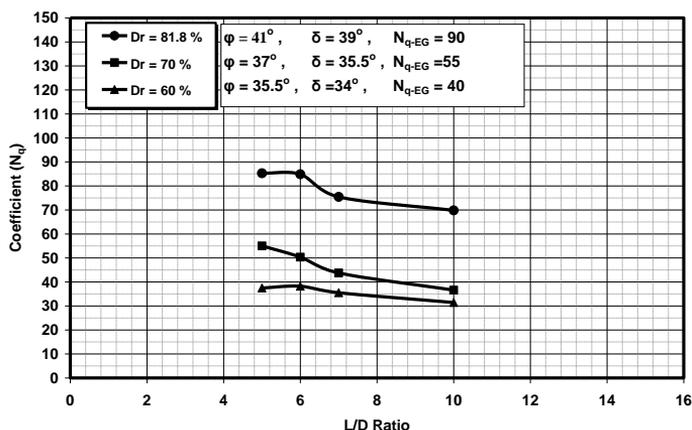
Figure 13. Relationship between coefficient ( $N_q$ ) and L/D ratio (O-cell tests)
