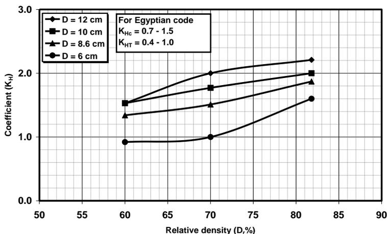
Figure 16. Relationship between coefficient ( $K_H$ ) and relative density (O-cell tests)
