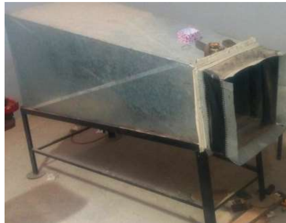
Fig. 14. Wind tunnel used for the evaluation of the power coefficient
