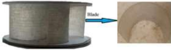
Fig. 7. The manufactured VAWT composite blade
