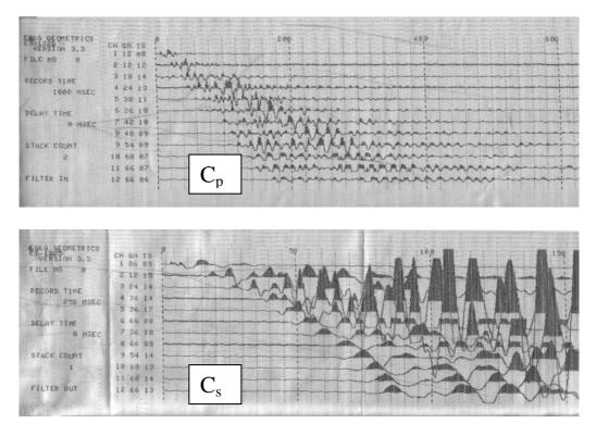
Fig. 2: A sample of the geophone recorded seismograms for arrival times using EG&G system.
