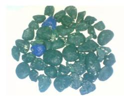
Figure (1): Coated aggregates with polypropylene
