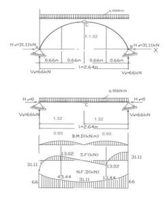
Fig. 3 Schematic diagram for a circular arch
