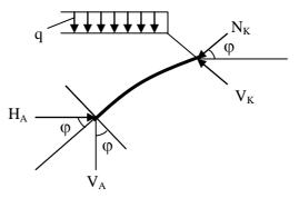
Fig. 4 Left hand section of the studied arch
