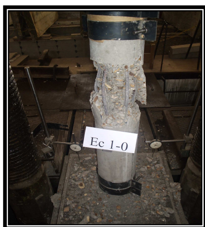
Photo (1) Final failure mode ( Bs 3-0 ). Photo (2) Final failure mode ( Es 1-0 ). ( The first mechanism )
