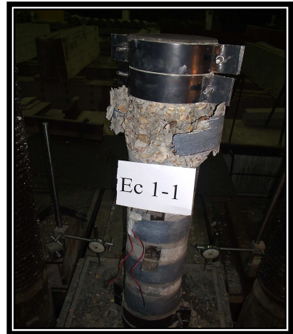
Photo (4) Final failure mode (Ec 1-1). (The second mechanism)
