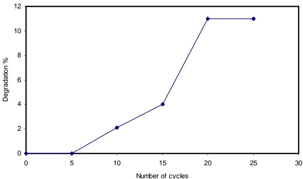
**Fig. (9) Relation between number of cycles and degradation % for -250 micron particle size of coal at 10 % solid concentration by wt..**
