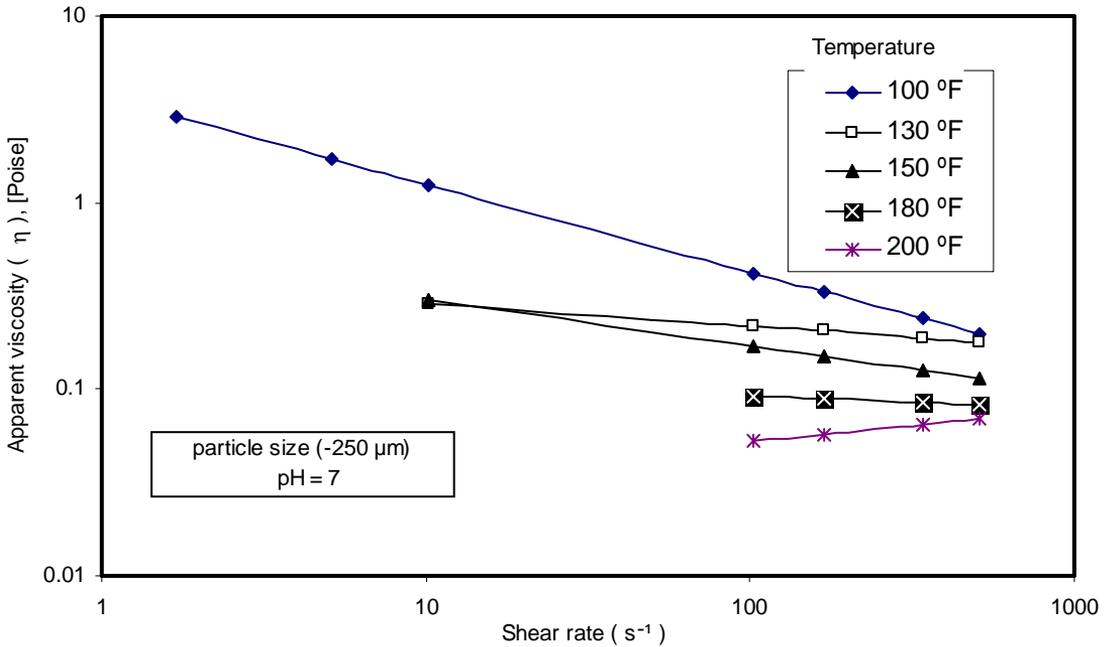
Fig. (4) Effect of trmperature on apparent viscosity for (-250  $\mu m$ ) particle size sample at 40% solid concentration by wt.
