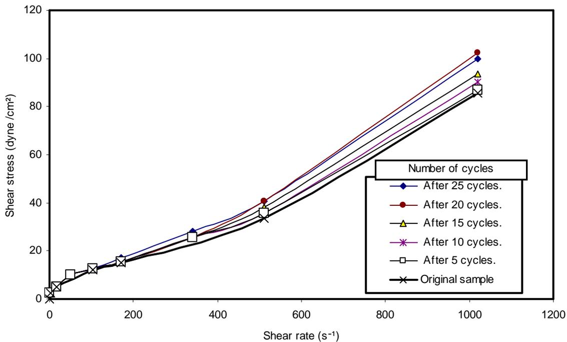
**Fig. (10) Relation between shear stress and shear rate for -250 micron sample at different number of pumping cycles (distance).**
