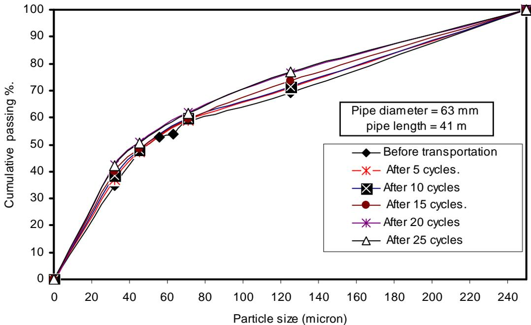
**Fig. (8) Particle size distribution for (-250 μm particle size) CWS before and after transportation.**
