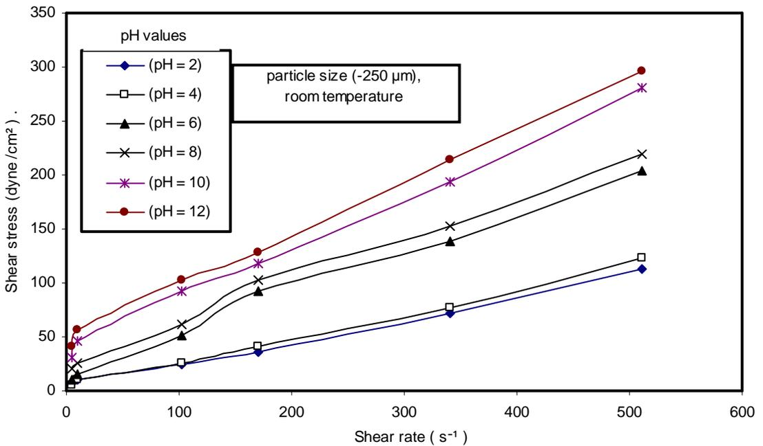
Fig. (5) Relation between shear stress and shear rate for (-250  $\mu m$ ) particle size sample at different pH, and constant solid concentration of 40 % by wt.
