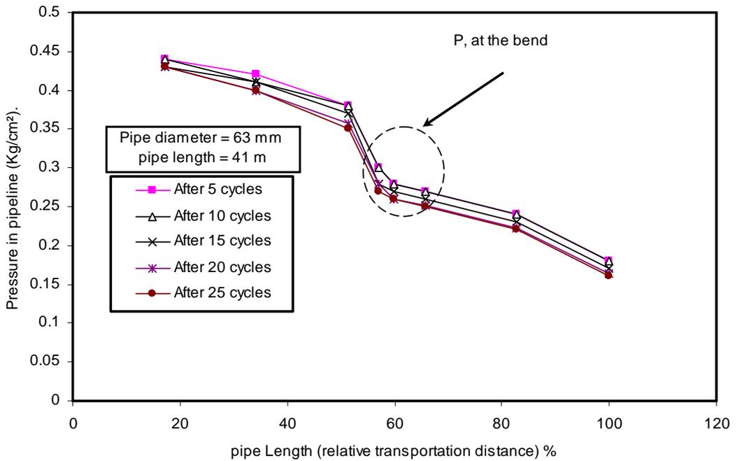
Fig. (12) Effect of transportation distance on pressure drop at different number of cycles for (-250 micron particle size) at 10 % solids by wt.
