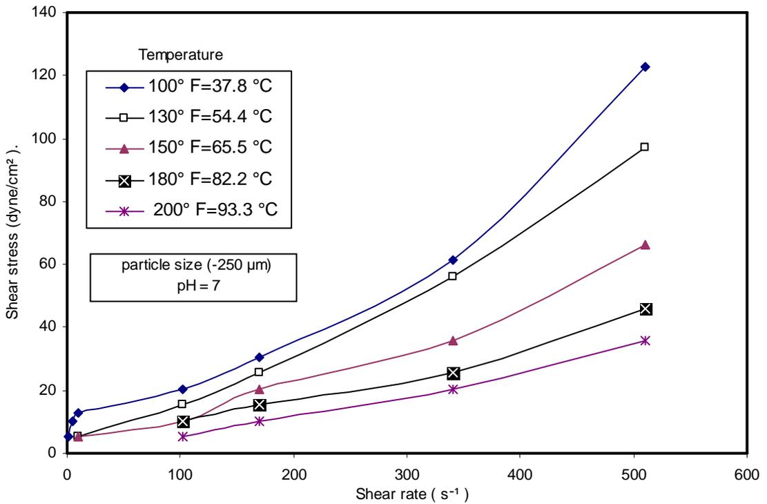
**Fig.(2) Relation between shear stress and shear rate for (-250 μm) particle size sample at different temperatures and constant solid concentration of 40 % by wt.**
