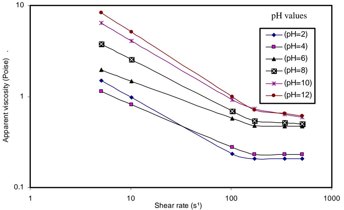
**Fig. (7) Effect of pH on apparent viscosity for (-250 micron) coal slurry sample at different shear rates and at constant solid concentration of 40% by wt.**
