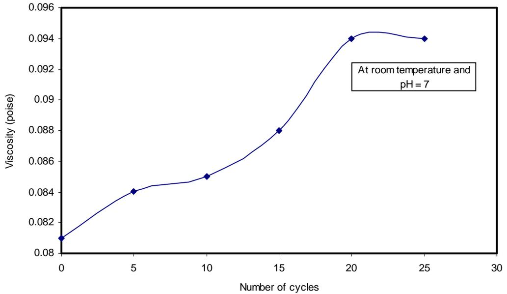
Fig. (11) Effect of number of cycles on viscosity of -250  $\mu\text{m}$  particle size sample at 10% solid concentration by wt..
