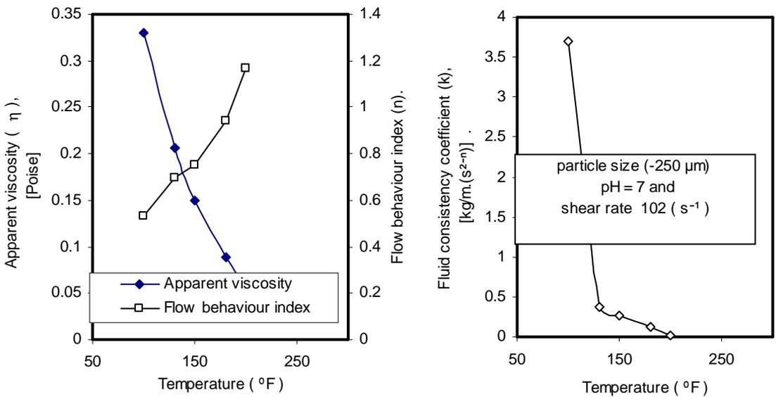
**Fig. (3) Effect of temperature on apparent viscosity and non-Newtonian parameters for (-250 μm) particle size sample at 40% solid concentration by wt. pH = 7 and shear rate 102 ( s<sup>-1</sup> )**
