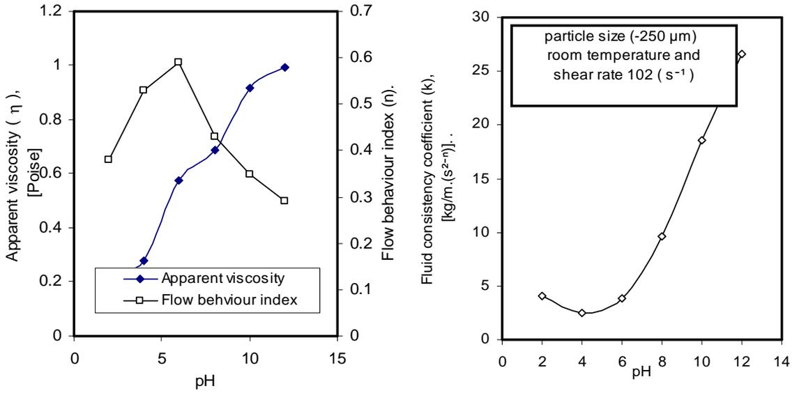
**Fig. (6) Effect of pH on apparent viscosity and non-Newtonian parameters for (-250 μm) particle size sample at constant solid concentration of 40% by wt. at shear rate 102 ( s<sup>-1</sup> ) and room temperature**
