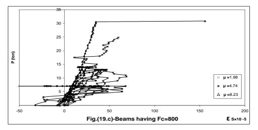
Fig.(19)-Load maximum concrete strain relationship for repeated loading and final static loading
