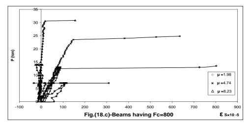
Fig.(18)-Load maximum steel strain relationship for repeated loading and final static loading
