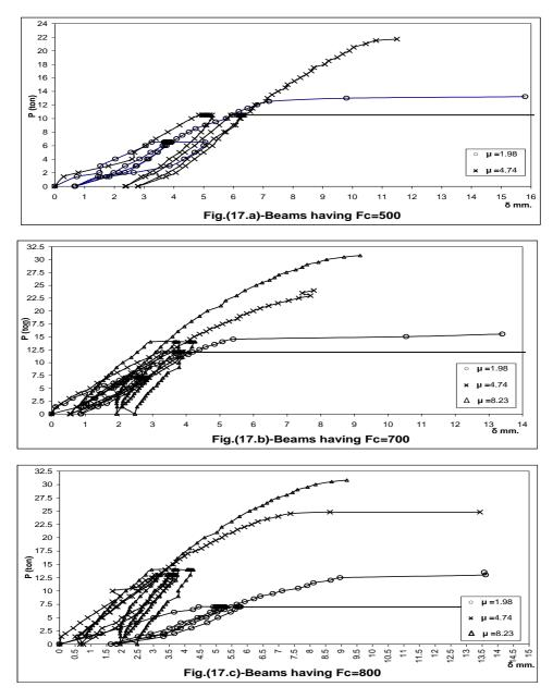
Fig.(17)-Load maximum deflection relationship for repeated loading and final static loading
