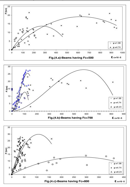
Figure (4) Load maximum concrete strain relationship for static loading
