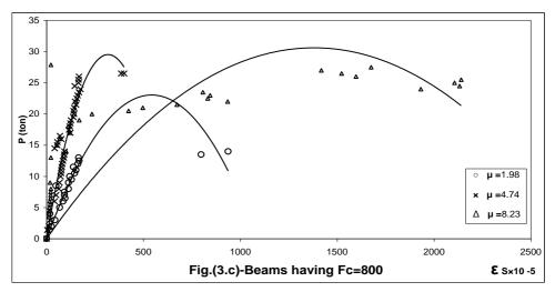
Figure (3) Load maximum steel strain relationship for static loading
