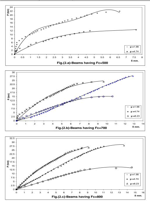
Figure (2) Load maximum deflection relationship for static loading
