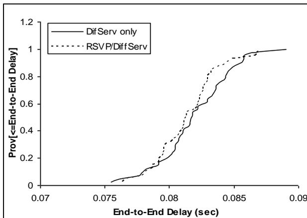
Figure 8 Cumulative distributions function for end-to-end delay for voice application
