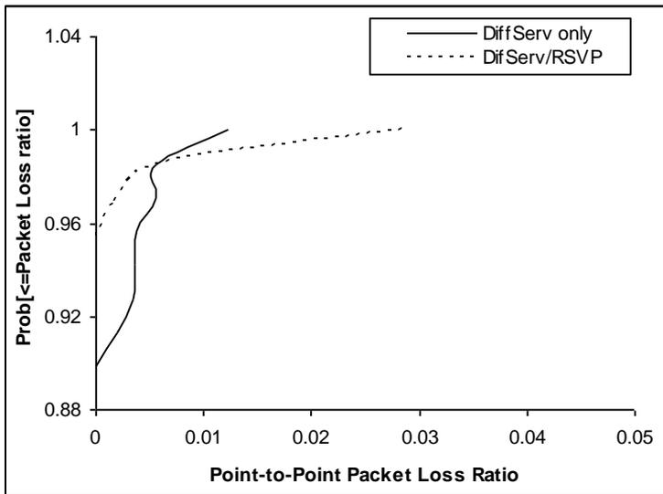
Figure 12 CDF for point-to-point packet loss ratio
