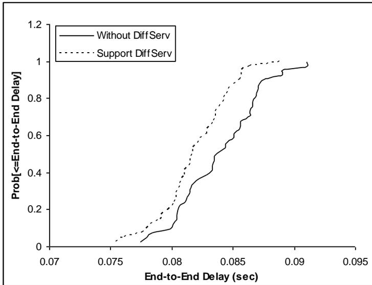
Figure 2 Cumulative Distribution Function for end-to-end Delay for voice application
