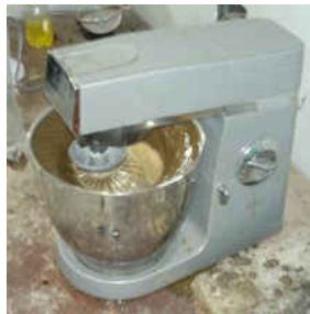
Fig. 5. mixing process of water and soap-stock
