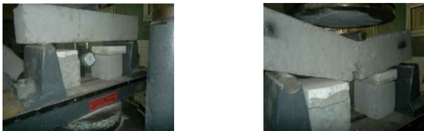
Fig. 8. flexural strength test.
