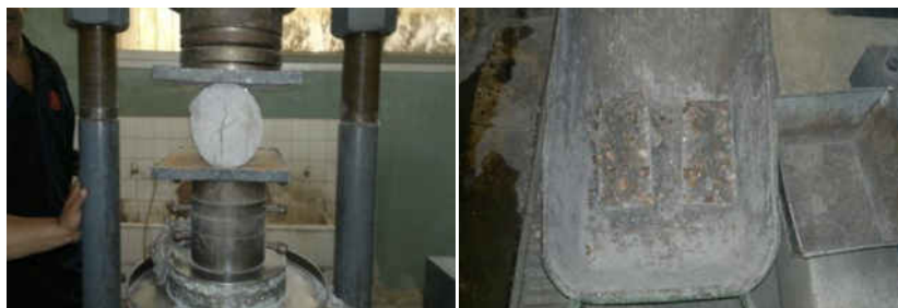
Fig. 6. Splitting tensile test.
