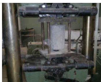
Fig. 7. Pull out bond strength test.
