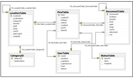
Fig. 6.Diagram showing the database relationship.
