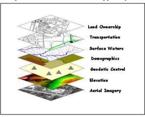
Fig. 4.Different types of layers provided by GIS [15].
