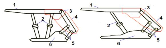
**Fig. 1.** The chock - shield supports & The 2-leg shield supports 1-canopy 2-hydraulic legs 3-side shield 4- goaf shield 5-lemniscate linkages 6-base
