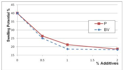
Fig. 14. Effect of additives on swelling potential
