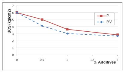
**Fig. 12.** Effect of additives on unc. comp. strength.
