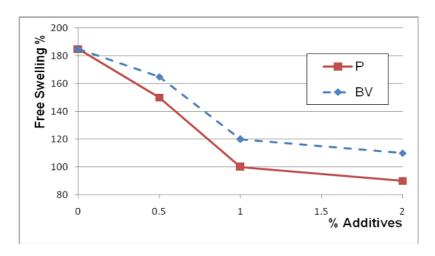
**Fig. 13.** Effect of additives on free swelling.
