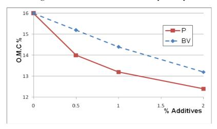
**Fig. 11.** Effect of additives on optimum water content.
