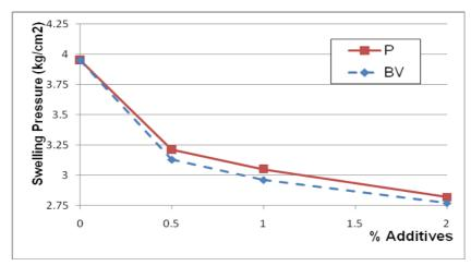
Fig. 15. Effect of additives on swelling pressure.
