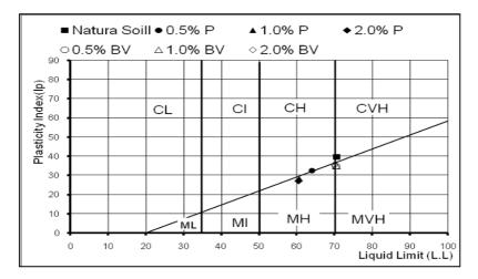
Fig. 4. Effect of additives on soil texture.
