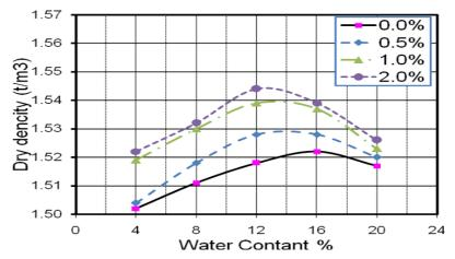
**Fig. 8.** Effect of Addicrete P on the compaction.
