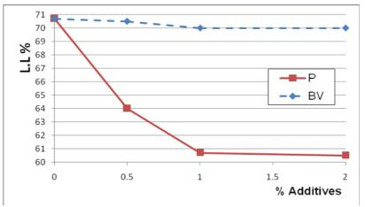
Fig. 5. Effect of additives on liquid limit.
