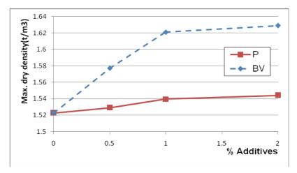
**Fig. 10.** Effect of additives on max dry density.
