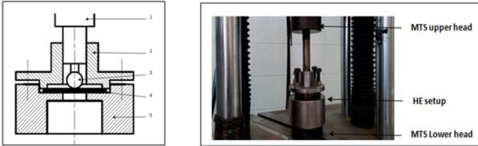
Fig. 5. The designed setup (left) and a photo of the MTS machine
