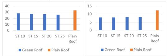
**Fig. 4.** Comparing Heating and Cooling Loads of Plain Roof and Green Roof With Deferent Soil Thickness (ST) (Left: Heating Load, Right: Cooling Load)
