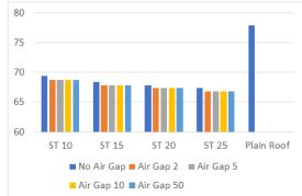
**Fig. 3.** Comparing EUI of Green Roof Performance for Deferent Soil Thickness (ST) and Air Gap With Plain Roof When Apartment is Facing South
