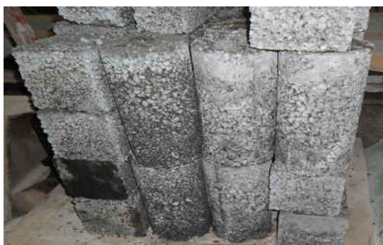
Fig. 11. The Appearance of Mixtures Prepared Using the EAFSS Fine and Coarse Aggregate
