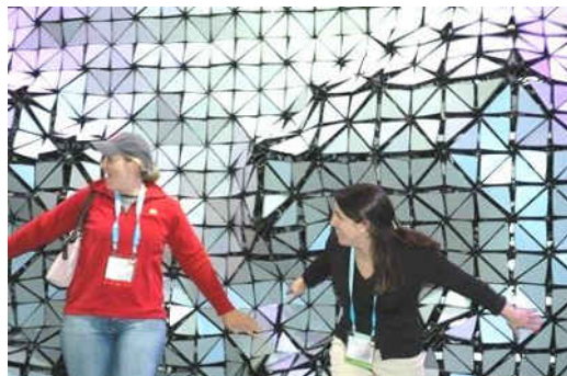
Fig. 15. HypoSurface is the World’s first display system where the screen surface physically moves! Information and form are linked to give a radical new media technology: an info-form device. [18]
