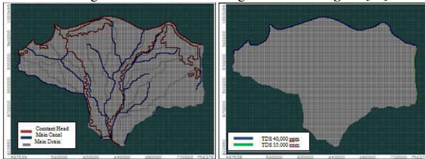
Fig. 8. Model Boundary Condition for (a) Head (b) Concentration
