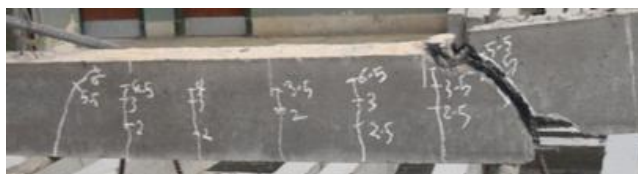
Photo 1. Mode of failure of beam (BF0).
