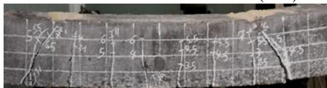
Photo 3. Mode of failure of beam (BF2).
