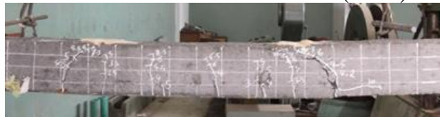
Photo 7. Mode of failure of beam (BFS2).
