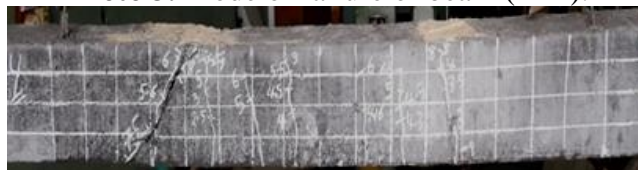
Photo 4. Mode of failure of beam (BF3).
