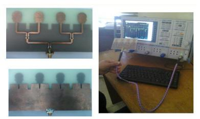
Fig. 39. The fabricated photos of the proposed 4 x1 UWB linear antenna array.
