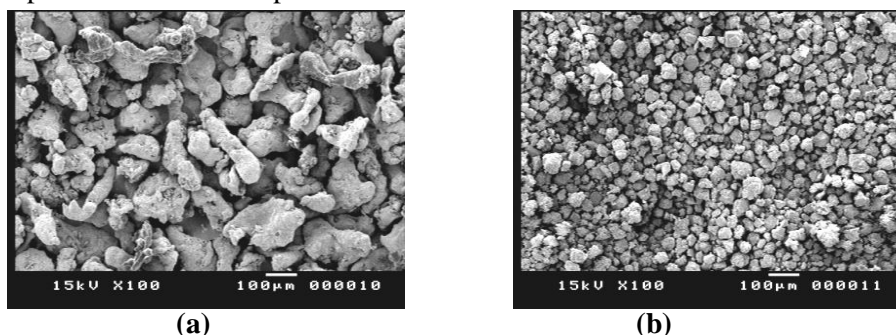
Fig. 6. SEM images for the as-received powders: (a) Aluminum (b) Alumina
