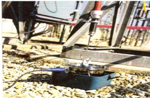
Fig. 2. Liquid insulation cell connected for testing.
