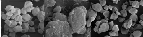
Fig (1): Native Starch as Scanning Electron Microscopy at Magnification 4000 Times.
